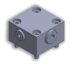
The Covers H9-LC\*S are designed to hold Hydronine make 2 port slip-in cartridge valves in the cavities machined as per ISO 7368. It also meant to connect port C of the Cartridge to one of the two pressure sources, brought to its port X and port Z1. Automatic selection of higher source pressure and isolation of these pressures from one another is done by the built in Shuttle valve in the cover.
