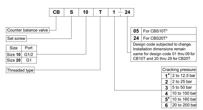
**Note** : Cracking pressure marked with **\*** are not available in CBS20T
