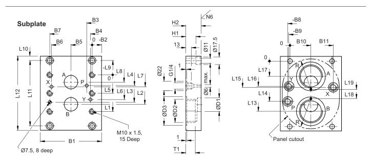
Use M10 x 1.5 x 40L  $\,$  S.H.C. screw 10.9 grade. Tightening torque 77 Nm.
